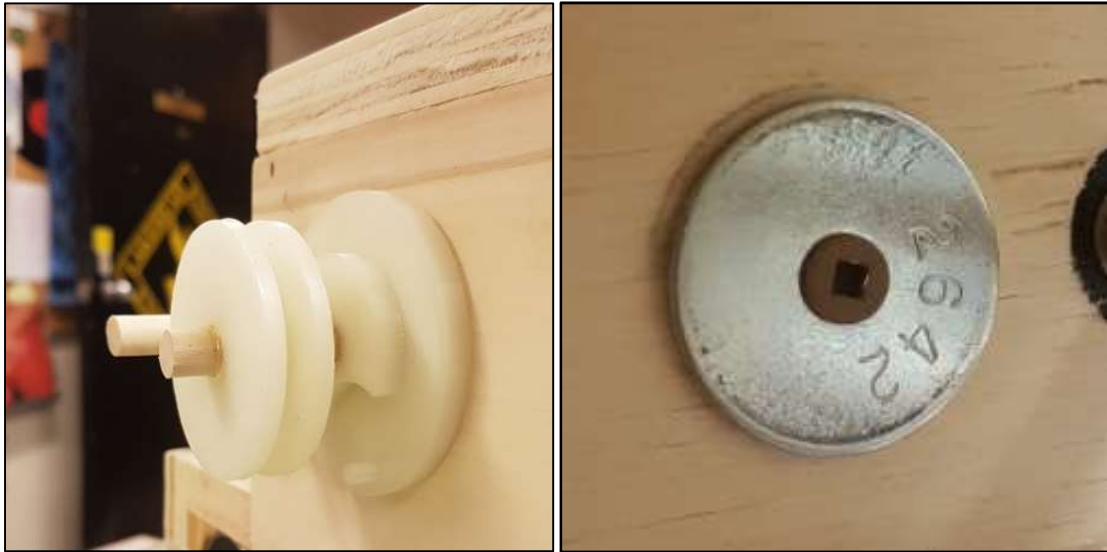
Figure 14: Reduced length dowel from outside (left) and inside (right)
